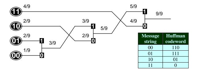
In this case the average number of bits required to encode each pair of message bits is
