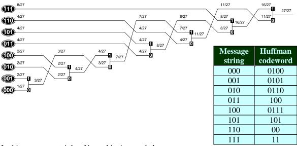
In this case every triple of input bits is encoded as
